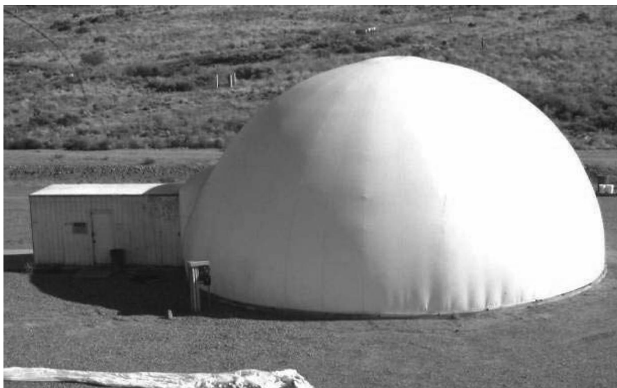
Fig. 1. 1000 m 3 explosive aerosolization chamber with a capacity of 0.23 kg of high explosive (Harper et al. 2006).
